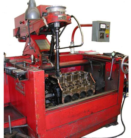
**Inboard Engine Block Honing**
