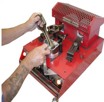
**Press Wrist Pins On and Off Rods**
