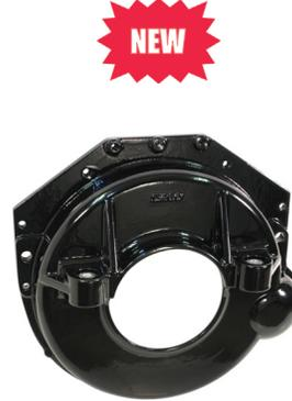
IMCO's new flywheel bellhousing is a direct replacement for installations using "Bravo" XR, XZ and IMCO X-Treme Advantage SC drives. The new bellhousing is reinforced in all critical areas with additional gusseting around the motor mount area. There is a flange at the top of the housing for accessory mounting. Better... and still affordable!
